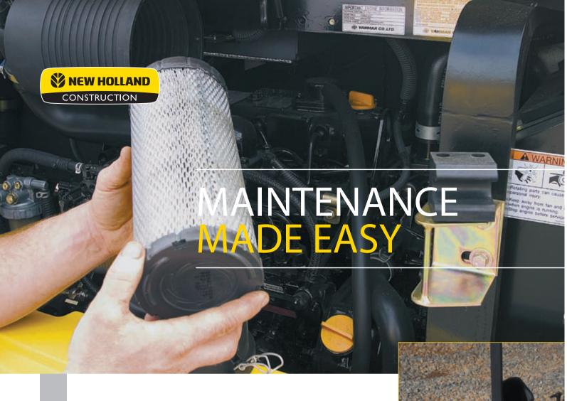
New Holland compact excavators are built with ease of maintenance in mind. Swing-open service doors and hinged access covers provide fast, easy access to maintenance points. And, there's no need to tilt or remove the canopy or cab to access the swing motor, boom swing cylinder and control valve. It's as easy as removing the appropriate guards.
