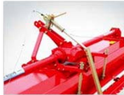
Central-spring pressure adjustment.
