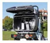
**GRASS COLLECTOR** WITH A REAL CAPACITY OF 1,000 LITRES and hydraulic tilting at a height of 210 cm.
