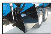
Hydraulically controlled wide slide tray with magnets for ground feeding.
