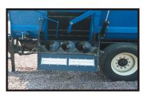
Auger discharge is hydraulically powered, height adjustable, includes magnets and delivers feed to bunks.
