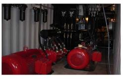
**Power Pack** is a self contained 750HP unit that eliminates the need for a separate power room or structure.
