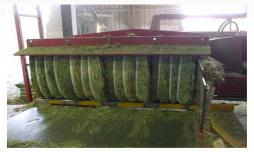
**Quarter Cut Bales** are created with an addition of a cutter box, which slices the 260lb bale into 4-65kg 3 tie bales.
